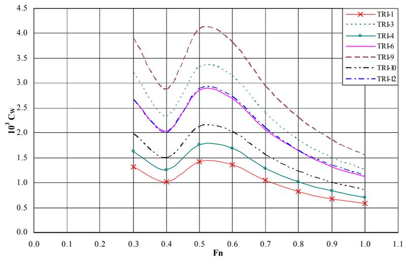
Figure 16: Wave Resistance Coefficients, SHIPFLOW,  $X/L_1$  -0.4
