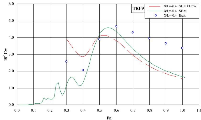
Figure 26: Wave Resistance Coefficients, Expt, SHIPFLOW and SBM, TRI-9, X/L=-0.4
