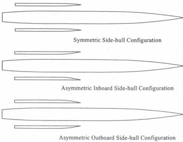
Figure 5: Model side hull configurations (Ackers et al (1997))
