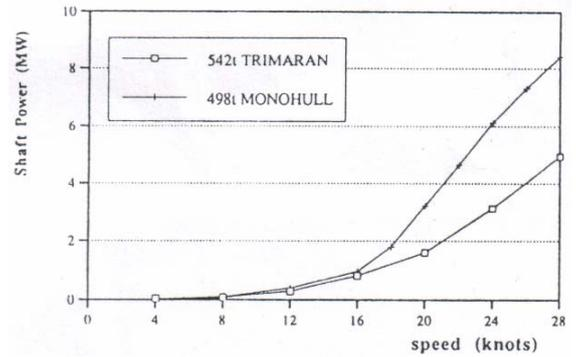
Figure 3: Shaft Power for mono-hull and trimaran offshore patrol vessels, Pattison and Zhang(1995)
