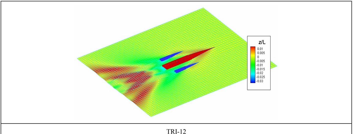
Figure 18: Wave Pattern, SHIPFLOW at  $F_n$  0.5 and  $X/L_1$  -0.2
