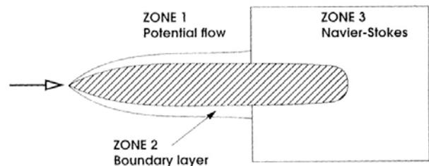
Figure 11: Schematic Diagram of SHIPFLOW Calculation Zone
