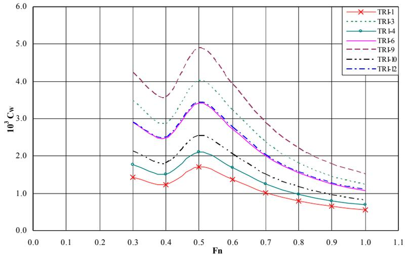
Figure 15: Wave Resistance Coefficients, SHIPFLOW,  $X/L_1$  -0.3
