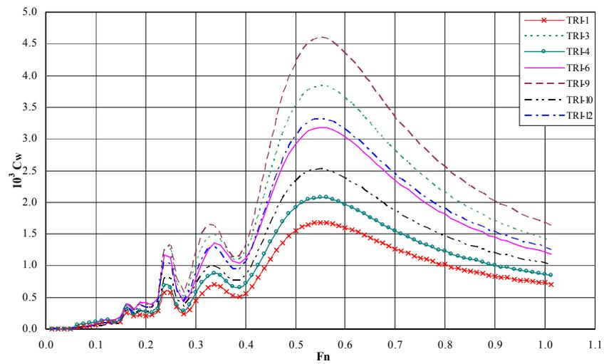
Figure 22: Wave Resistance Coefficients, SBM,  $X/L_1$  -0.4
