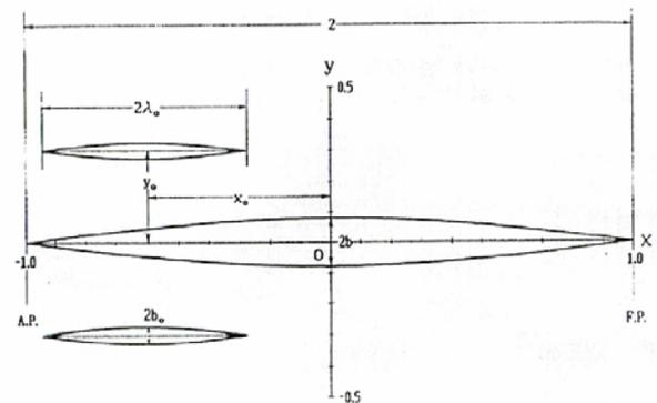
Figure 6: Trimaran Coordinate System, Suzuki & Ikehata (1993)
