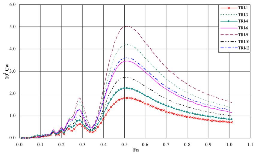
Figure 21: Wave Resistance Coefficients, SBM,  $X/L_1$  -0.3
