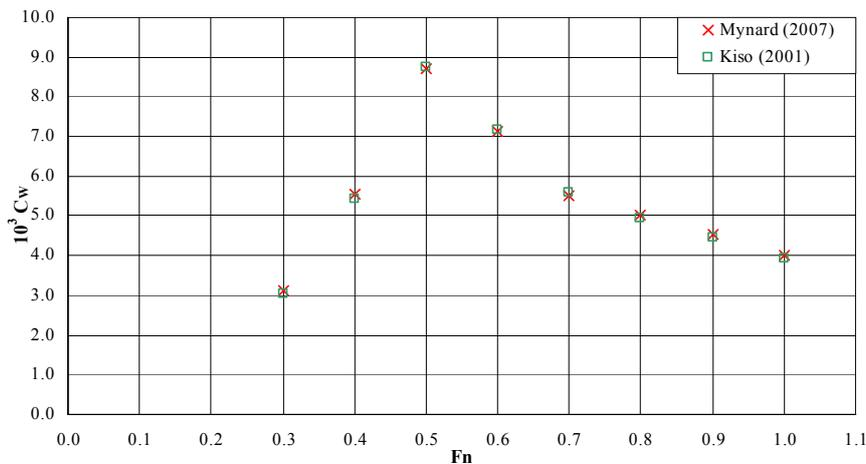
Figure 12: Comparison between Tank Testing Results, TRI-9, X/L<sub>1</sub> -0.2
