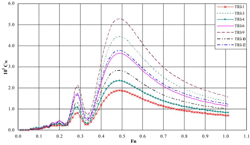
Figure 20: Wave Resistance Coefficients, SBM,  $X/L_1$  -0.2
