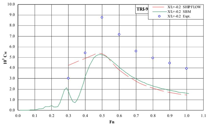
Figure 24: Wave Resistance Coefficients, Expt., SHIPFLOW and SBM, TRI-9,  $X/L=-0.2$
