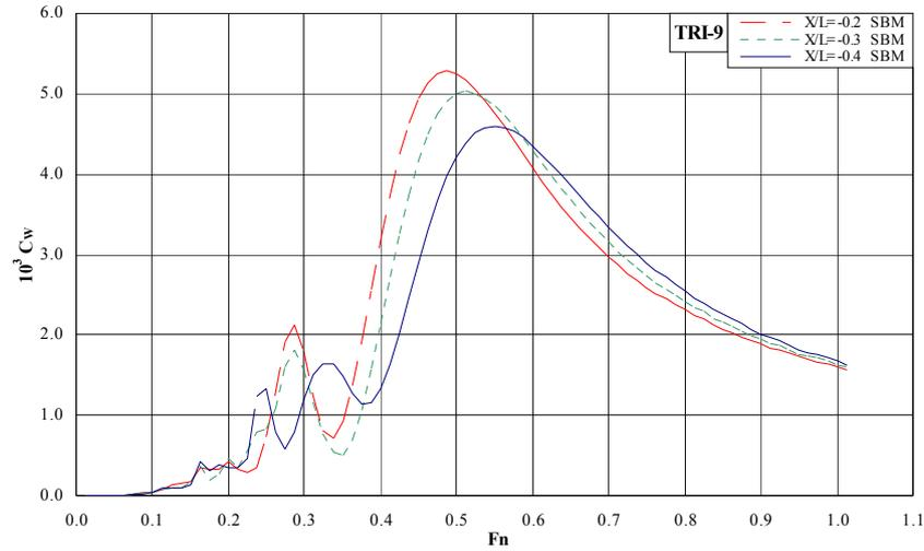
Figure 23: Wave Resistance Coefficient, Slender Body Method, TRI-9,  $X/L_1$  -0.2, -0.3, -0.4
