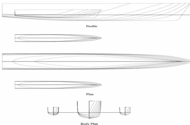
Figure 11: Configuration of Model 9 as a Trimaran
