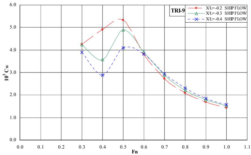
Figure 17: Wave Resistance Coefficient, SHIPFLOW, TRI-9,  $X/L_1$  -0.2, -0.3, -0.4
