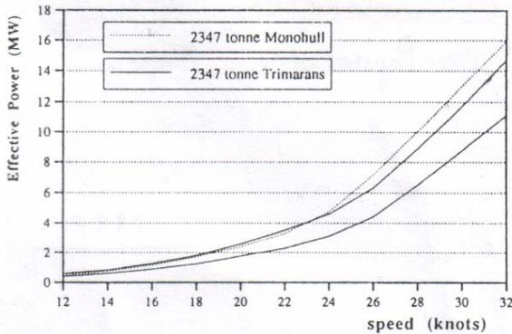
Figure 2: The effective power of a trimaran and mono-hull of the same displacement, Pattison and Zhang(1995)
