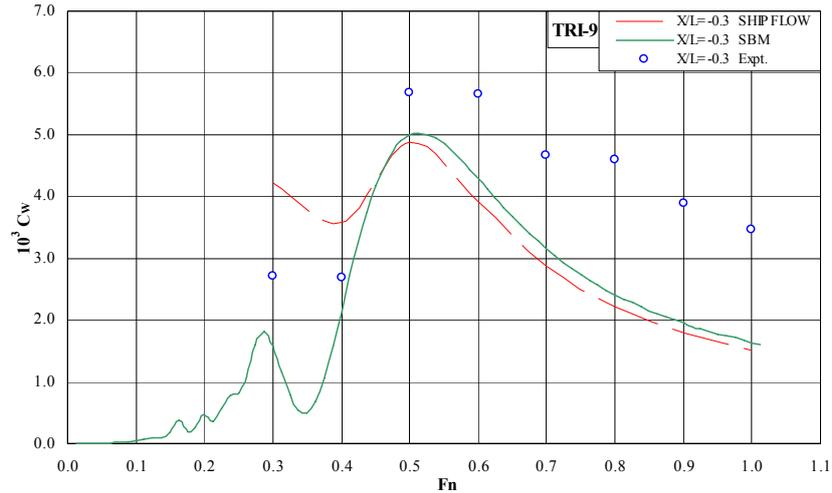
Figure 25: Wave Resistance Coefficients, Expt., SHIPFLOW and SBM, TRI-9, X/L=-0.3
