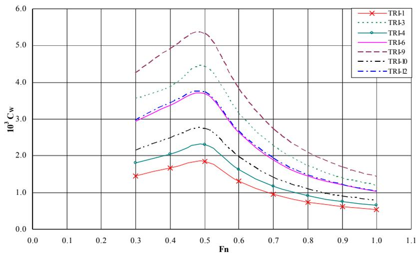
Figure 14: Wave Resistance Coefficients, SHIPFLOW, X/L<sub>1</sub> -0.2
