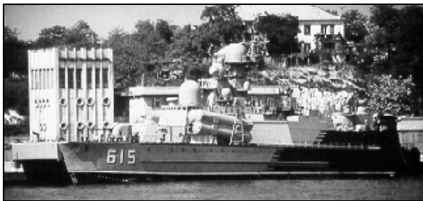
Figure 22. Russian 650-Ton Dergach Combatant SES (Canadian Forces Photo Courtesy of Guide to the Soviet Navy )
