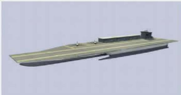
With 35 knots wind over deck and an 1100 ft flight deck, the ship is large enough for the C-130J to launch with a 40,000 lb payload and fly a 300 nm radius mission.
