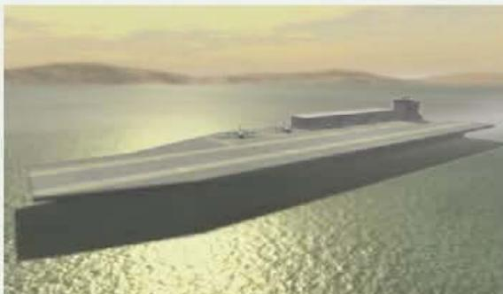
Preliminary analysis shows we can land the C-130J at 120,000 pounds on the HALSS deck with adequate margins. This weight is consistent with the scenario previously described.
