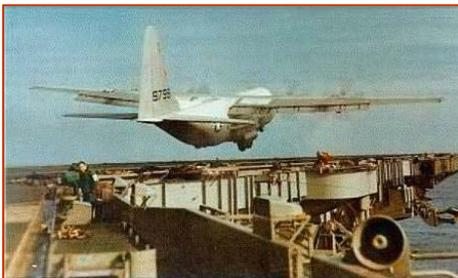
In 1963 launching and landing of C-130 was successfully tested onboard the USS FORRESTAL.
