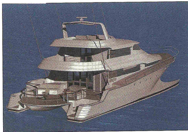
Forward and aft views of the Loomes-designed, long-range, 26.7m (87 1/2') wave-piercing catamaran shown under construction earlier in the article. The sportfisherman's 10m (32') beam permits an expansive interior volume, while the radiused, opera-style cockpit puts the angler close to the action, despite the size of the boat.
