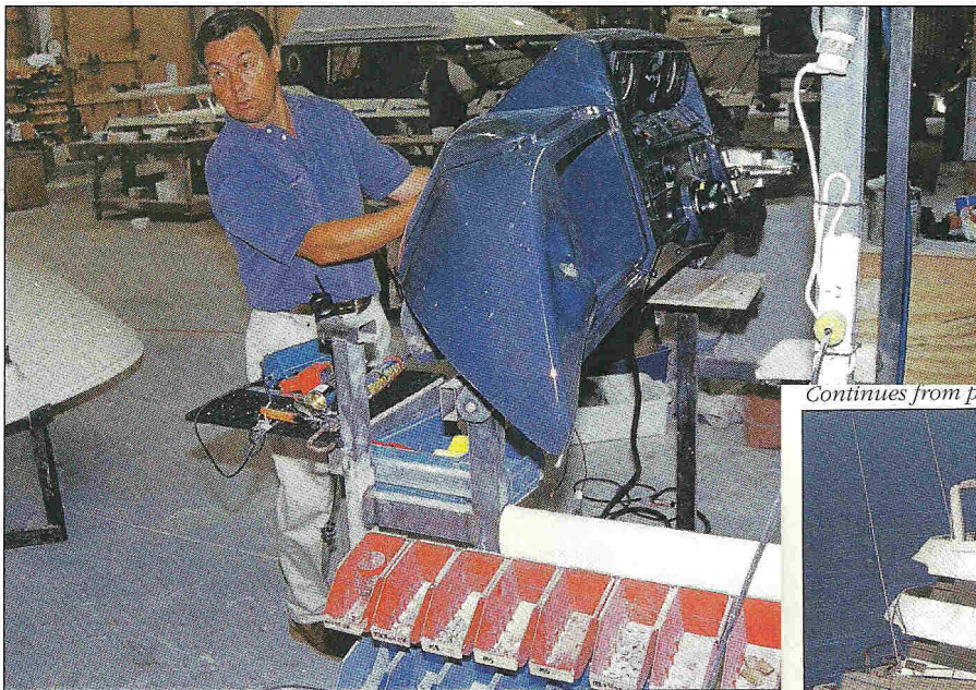
The McDell shop floor is arranged in automotive-style work cells, each one well-illuminated. Facing page —McDell's Ken Olson describes the various pieces of information posted at a workstation bulletin board; note the photos of typical manufacturing defects to be avoided. Left —Olson demonstrates the ease with which a worker can assemble both sides of an instrument panel.
