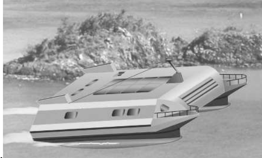
Fig.8. Semi-planing SWATH as a mini-ferry, 50 passengers, 30 kts.
