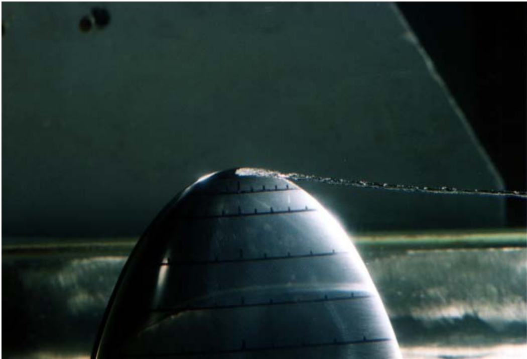
Cavitation on a Submarine Nose
