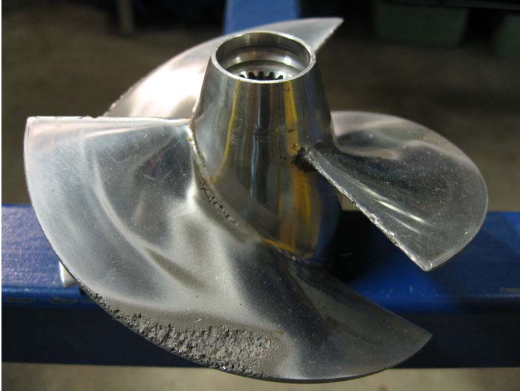
Cavitation in Propeller
