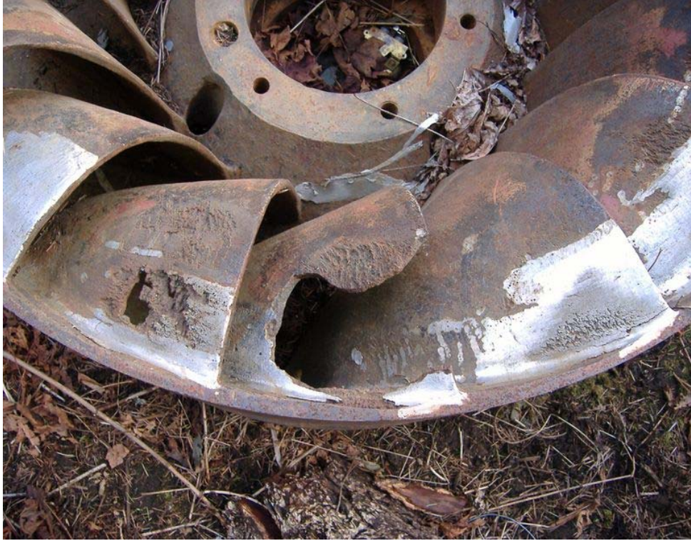
Cavitation in Francis Turbine Blade
