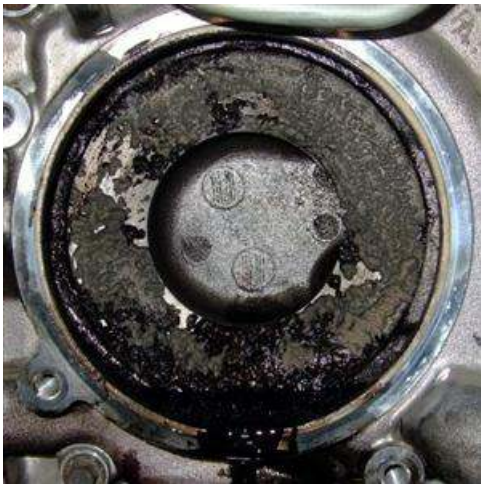
Figure 7: A cavitation eroded water pump cover from a 6.4L Ford Power Stroke diesel engine [5].
