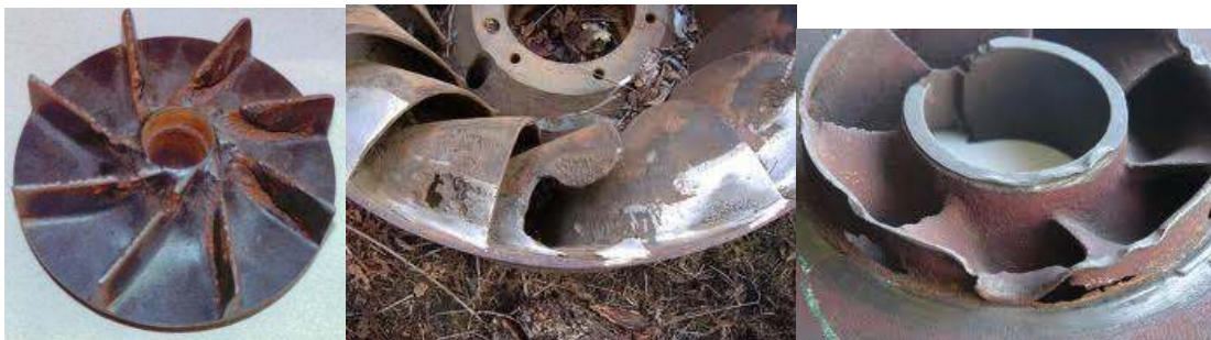
Figure 8: Cavitation damage in some pumps. Note the tag team effect caused by erosion and corrosion.
