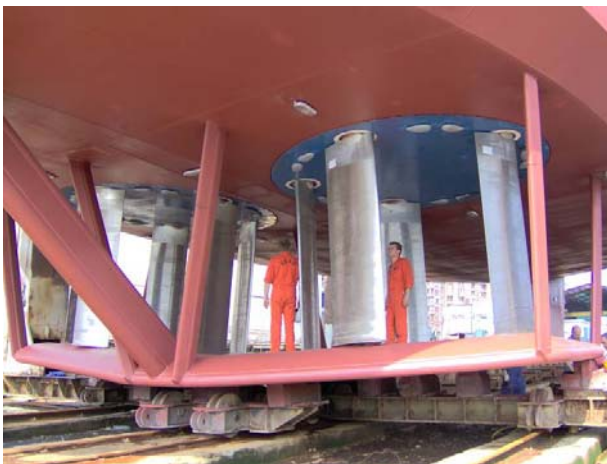
Fig. 2: Two VSP installed in a Voith Water Tractor and the thrust plate (propeller guard)
