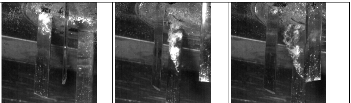
Fig. 19: Cavitation observation, n_M = 5 \text{ s}^{-1} , V_M = 0.473 \text{ m/s} , \lambda = 0.15 , K_{SX} = 0.490 , K_D = 0.426 , \sigma_n = 3.36
