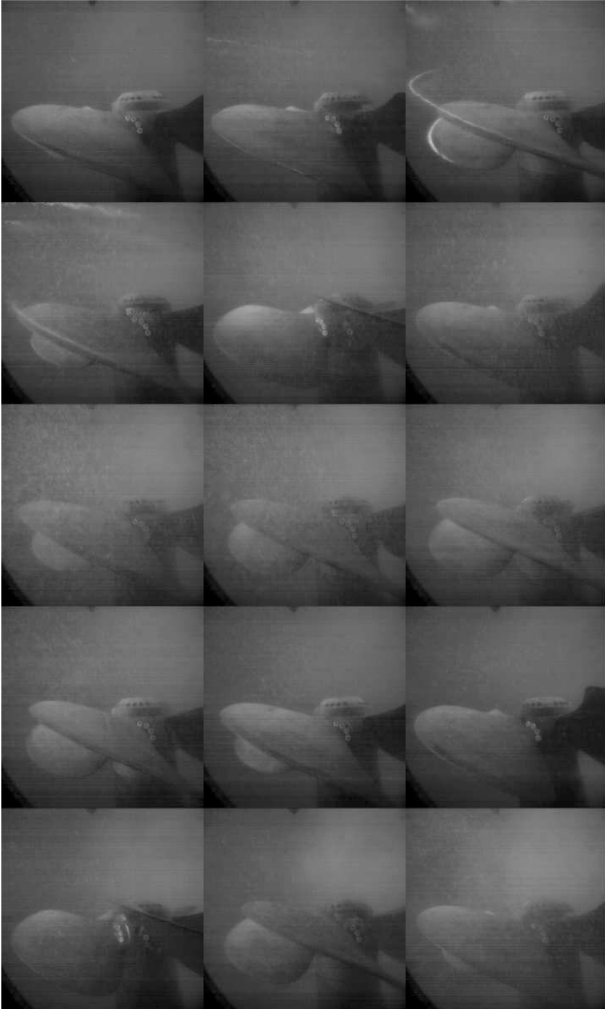
Figure 9.39: Cavitation behaviour of new PCS during deceleration, display interval 1s, start at t = 305s
