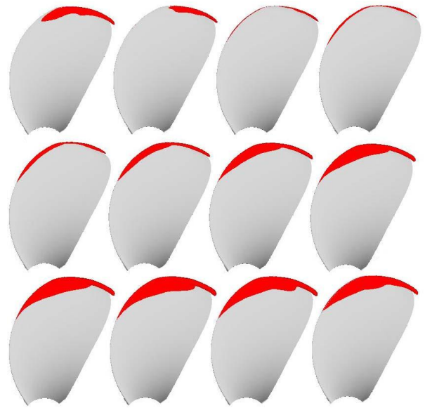
Figure 12 Cavitation profile on the conventional propeller at \varphi = 0^\circ - 330^\circ with 30^\circ intervals (from top-left corner to bottom-right corner) from the computation for \sigma_N = 2.2 in the behind-hull condition
