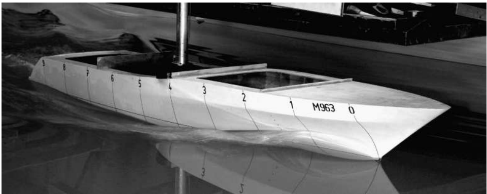
Figure 3.10. Model resistance test. Photograph courtesy of WUMTIA and Dubois Naval Architects Ltd.
