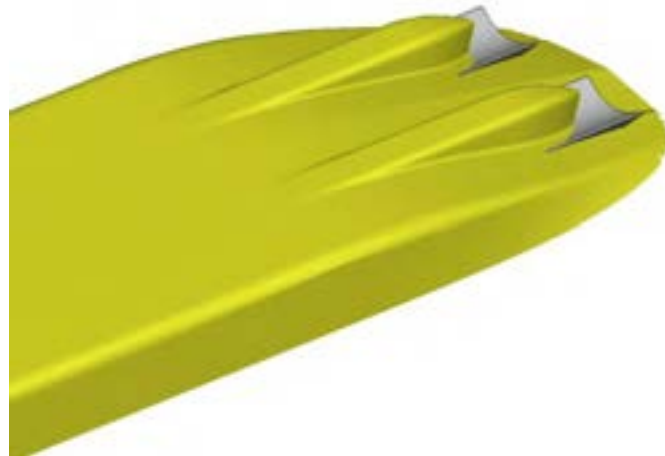
Figure 4. Aft view of the model ship with tunnels. Tunnels haven't been included in calculations.
