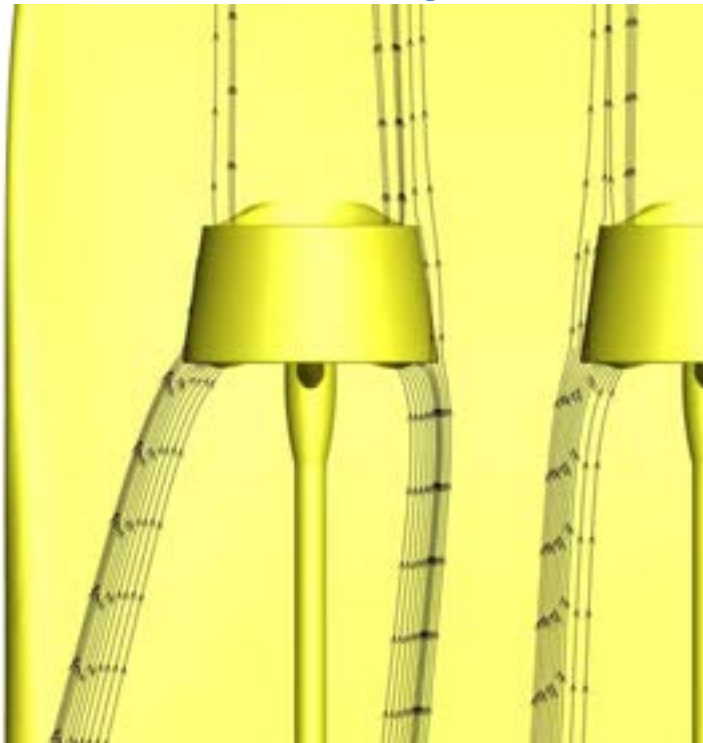
Figure 9: Propulsion computations; streamlines along the edge of the nozzle, note the high contraction of the flow at the inlet of the nozzle.
