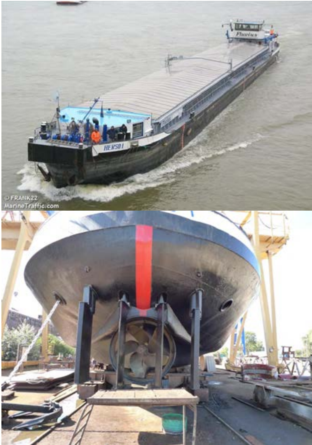
Figure 2: Ship (Herso-I): Entire ship and aft ship arrangement
