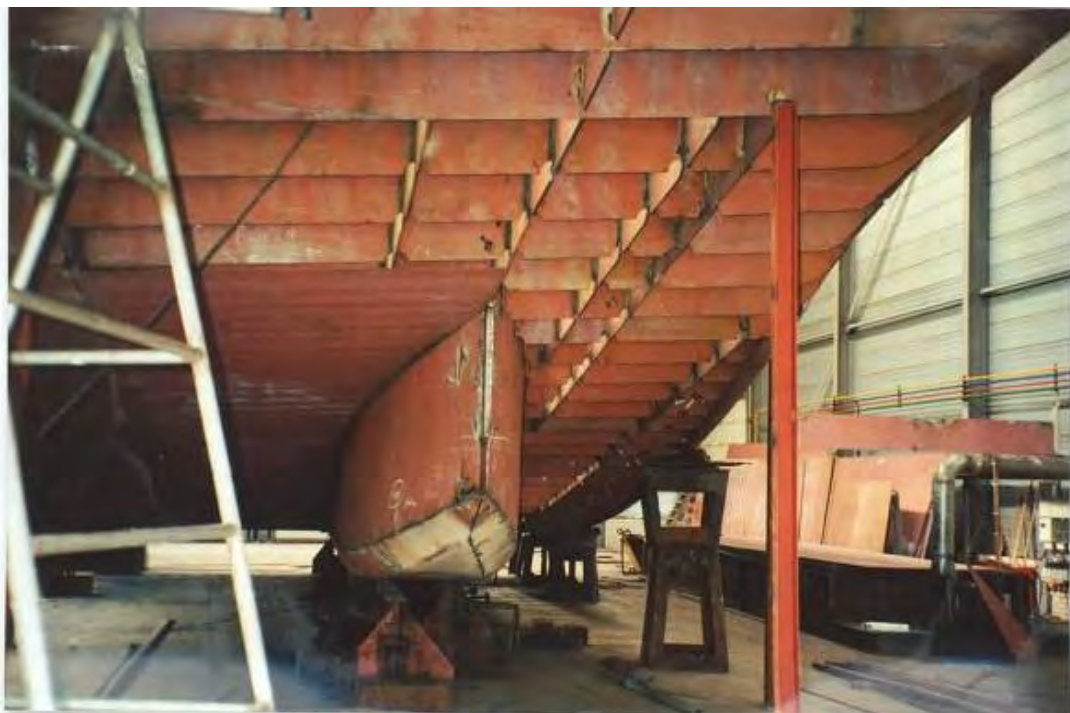
Figure 3. Aft view of the ship. Above: Tunnels and propeller nozzle. Down: Starboard gondola of the ship.
