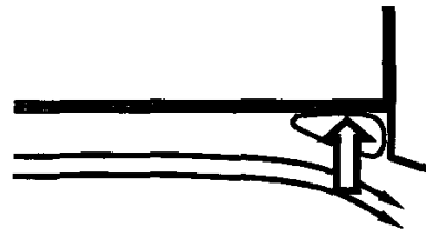
Fig.10. Schematic drawing of the integrated interceptor and stern flap.
