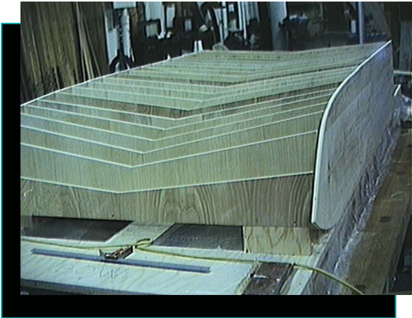
Calculated variation of deadrise to achieve maximum lift to drag ratio
