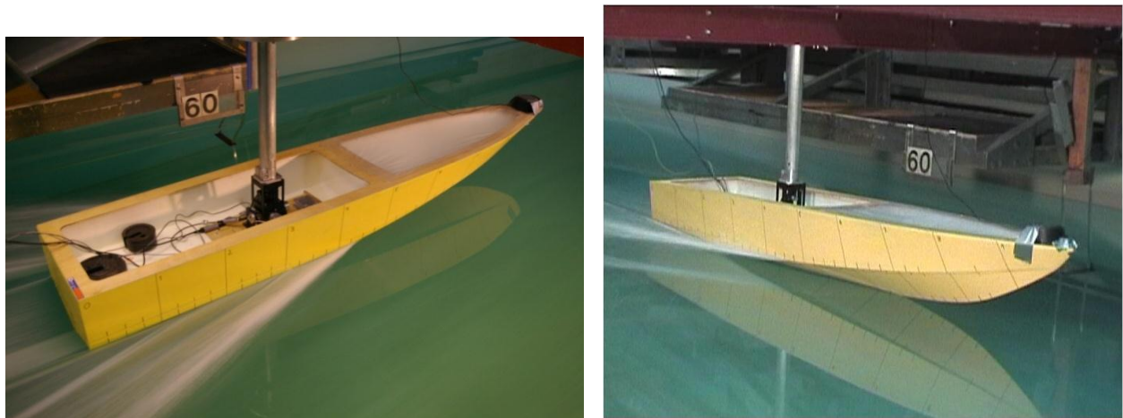
Figure 4: Example of a pair of photographs used to determine the wetted length. The image on the left is used to identify the position where the spray crosses the chine, and the image on the right is used to identify the position where the water contacts the keel. Run shows model C at a speed of 12.05 m/s.
