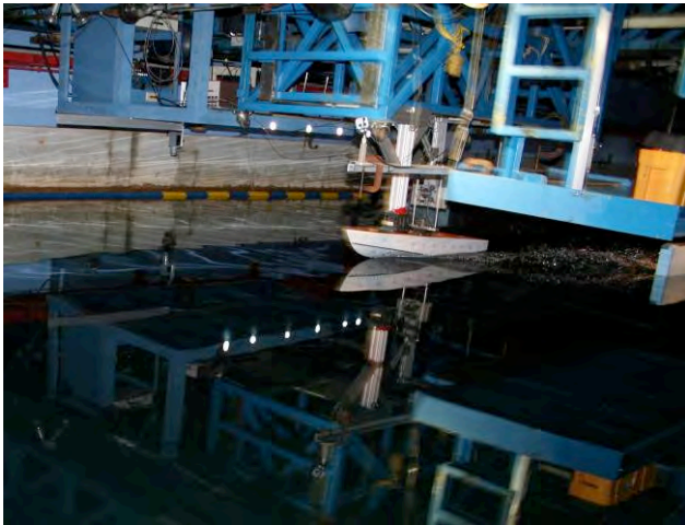
Fig. 7. Unstepped Hull running at 25 ft/s.
