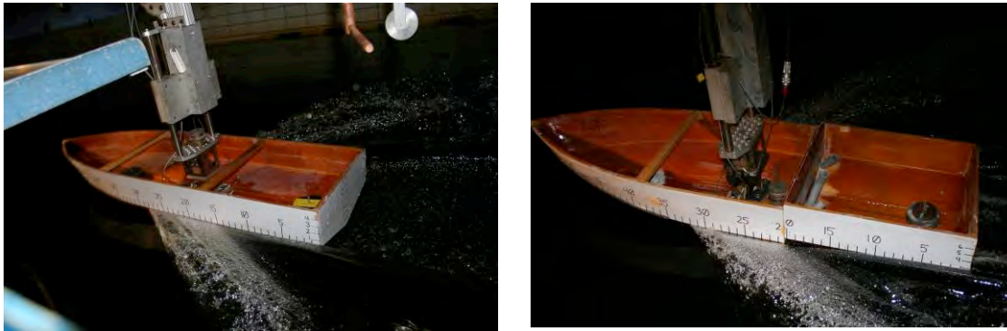
Fig. 6. (a) Unstepped Model @ 25 ft/s. (b) 0.696" Step Model @ 25 ft/s.
