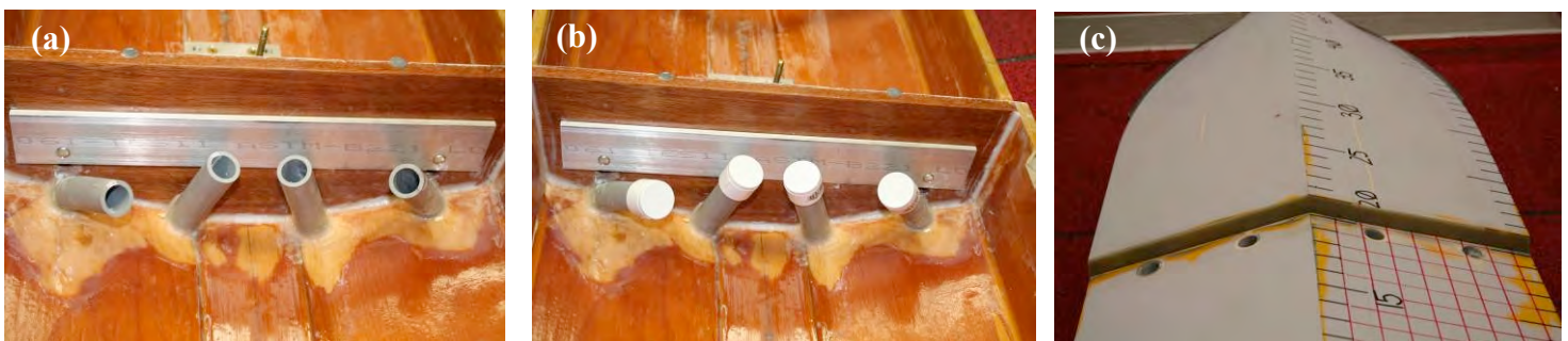
Fig. 4. Ventilation Tubes aft of step. (a) 100% open. (b) 0% Open. (c) Holes in hull bottom aft of step.
