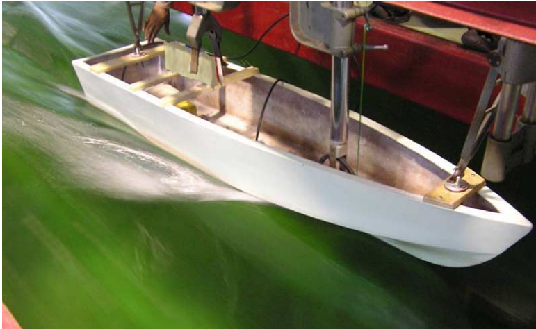
Fig. 14. Planing hull model in towing test condition.
