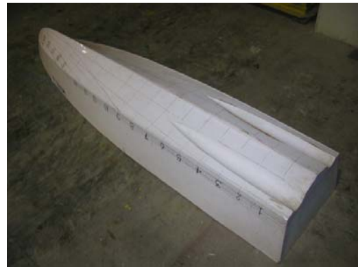
Fig. 7 Photograph of planing hull model
