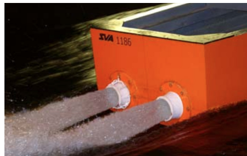
Figure 4.7 Model scale ATHENA with working waterjets [40]
