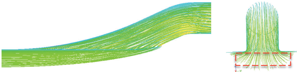
Figure 3.4 Backward tracing of the streamlines for obtaining the capture area; left: side view and right: stern view. The dashed line shows the rectangular capture area.
