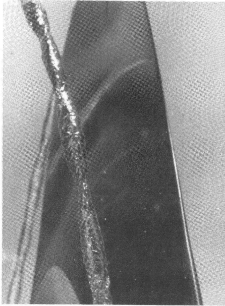
Fig. 8.11. Example of varying core radius (Propeller V blade 4 at J = 0.7 , \sigma_n = 2.0 , Re_n = 1.38 \times 10^6 )
