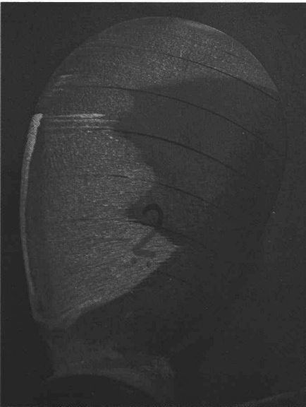
PLATE 3.15. PAINT PATTERN ON PROPELLER S AT J=0.4 . Re_n = 1.1 \times 10^6 .
