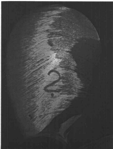
PLATE 3.11. PAINT PATTERN ON PROPELLER B AT J=0.4 .
