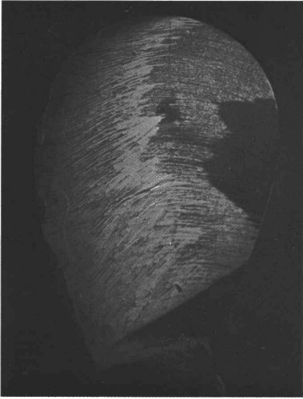
PLATE 3.14. PAINT PATTERN ON PROPELLER S AT J=0.6 .
