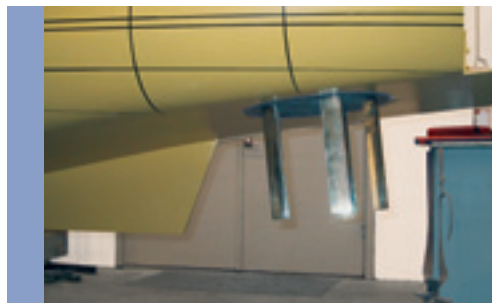
Fig. 7: Position of VSP in the stern of the PSV model. Propulsion: VSP size 32 R5
