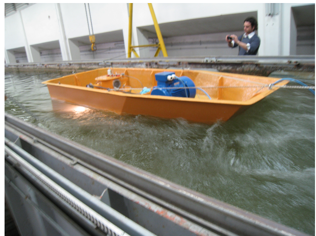
Figure 17 : Bollard pull tests in the towing tank.
