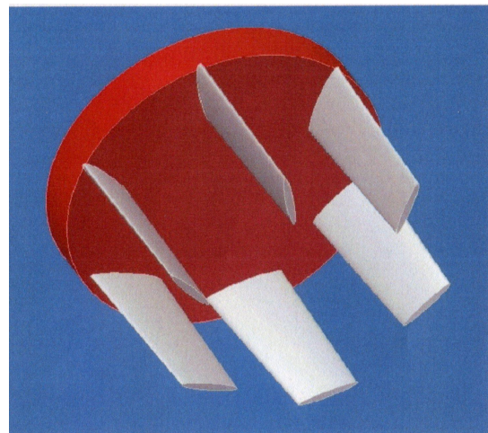
Figure 6 : Blades on a single impeller
