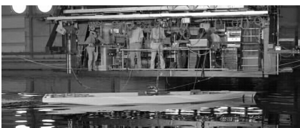
Fig. 28: Scale maneuvering tests with VCR for 100 m research vessel
