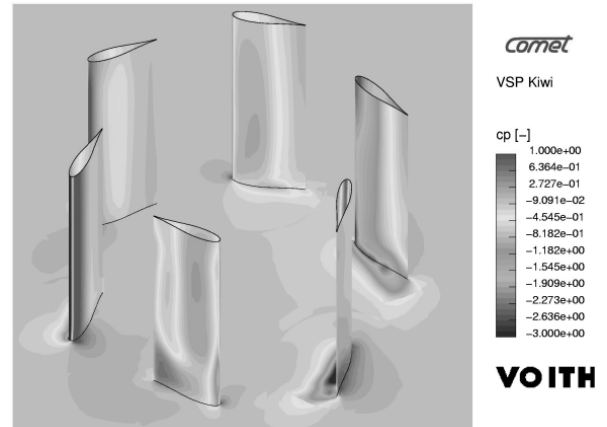
Fig. 6: CFD calculated pressure distribution on 6-bladed VSP
