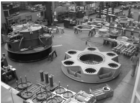
Fig. 5: Assembling a 6-bladed VSP in the workshop
