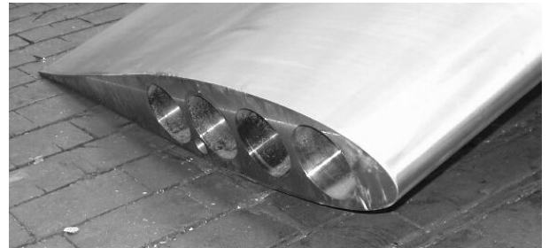
Fig. 14: VSP blade as build with weight reduction holes
