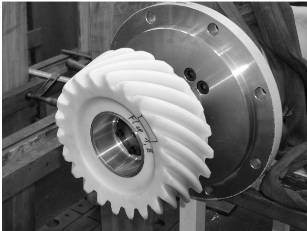
Fig. 20: Non-metallic pinion in development
