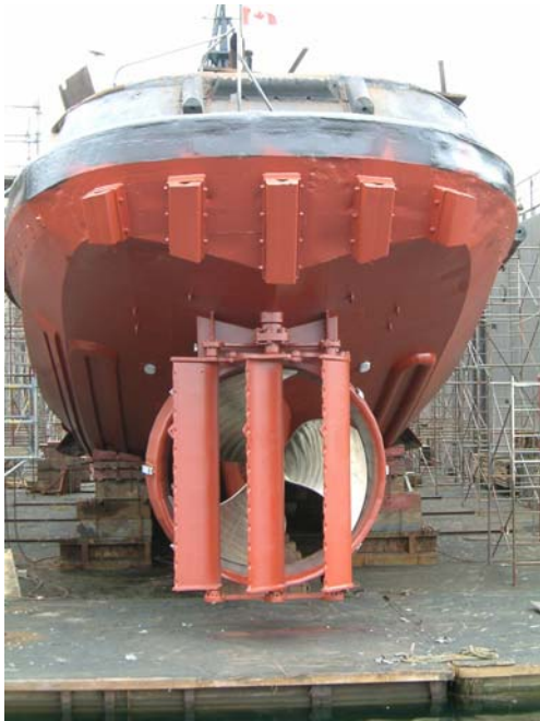
Figure 40. Neva Straights fitted with a high efficiency nozzle and rudders for barge pushing
