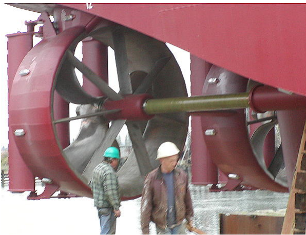
Figure 36. Phyllis Dunlap with high efficiency nozzles and stators
