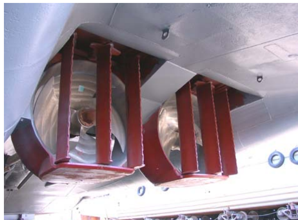
Figure 45. Pushboat Edgar Kotokak starboard side with integrated nozzles and steering units
