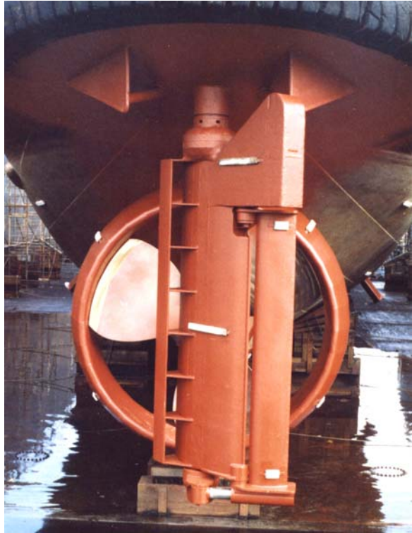
Figure 22. M.V. Larain nozzle installation
