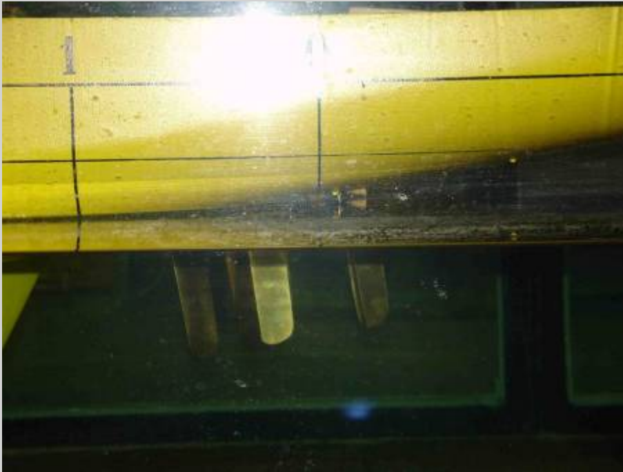
VSP is not running , the blades are partly in air
