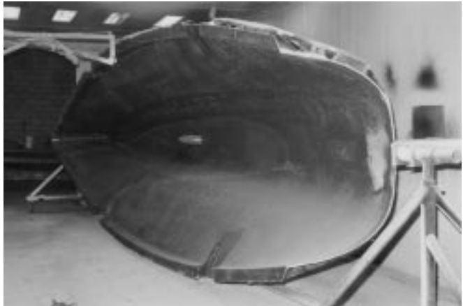
Figure 5-4 Production Female Mold on Spindle at Corsair Marine [author photo]
