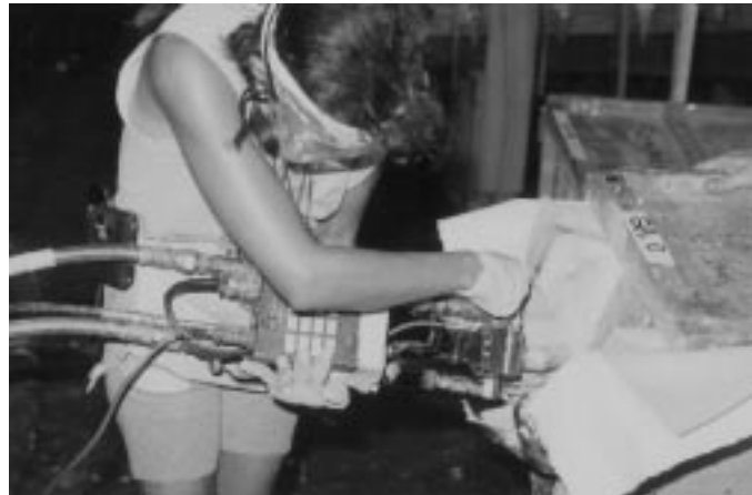
Figure 5-48 Two-Part Expansion Foam is Injected into Stringer Molds at Compsys with Careful Monitoring of Material Flow rate and Duration [author photo]
