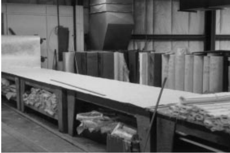
Figure 5-15 Material Layout Table at Heisley Marine [author photo]
