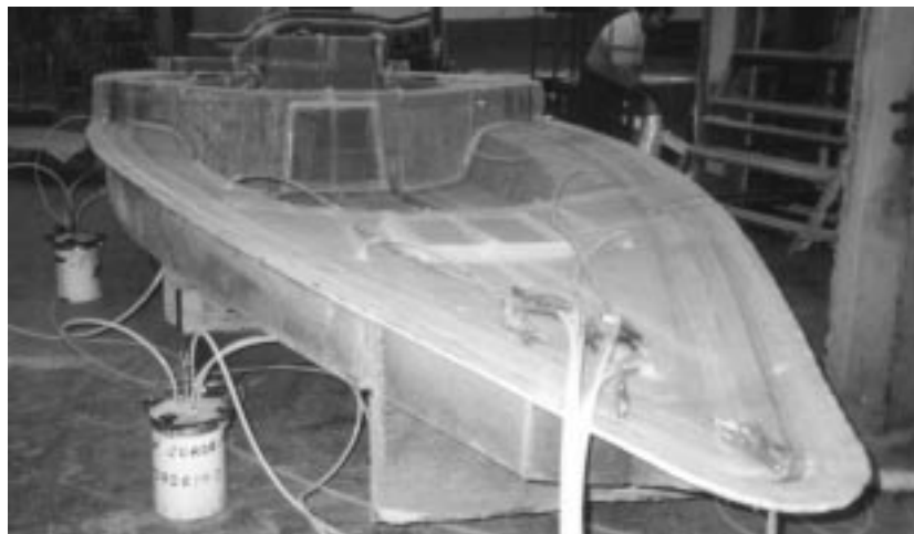
Figure 5-36 SCRIMP sm Infusion Arrangement [Mosher, TPI]
