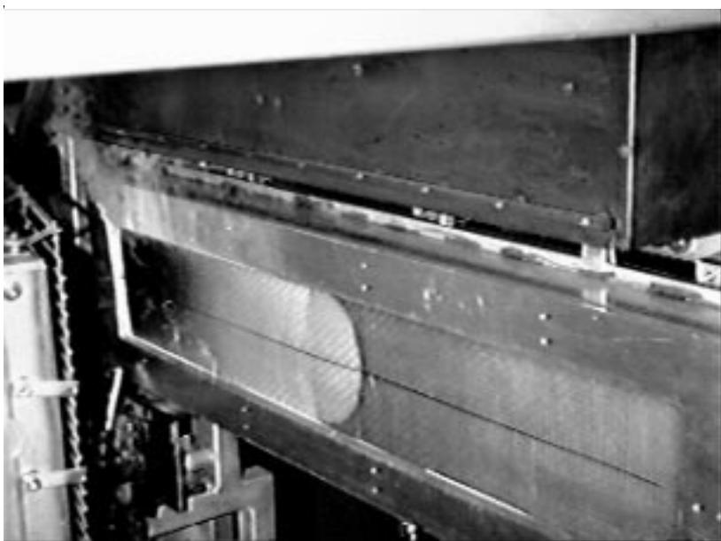
Figure 4-39 LIFT Test Panel at the Time of Ignition
