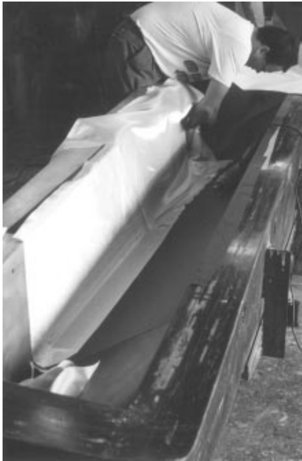
Figure 5-40 Prepreg Material is Positioned in Mold at Ron Jones Marine [author photo]
