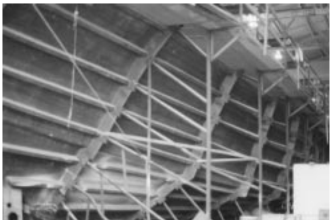
Figure 5-5 Metal Stiffened Female Mold at Northcoast Yachts [author photo]
