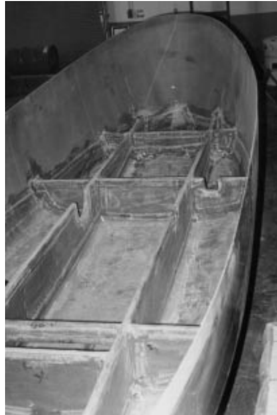
Figure 5-37 SCRIMPed sm U.S. Coast Guard Motor Lifeboat Built by OTECH [author photo]
