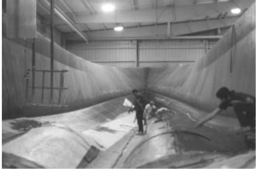
Figure 5-30 Laminators Consolidate Reinforcement Material Applied by Impregnator at Westport Shipyard [author photo]
