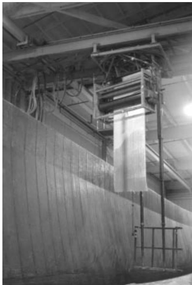
Figure 5-28 Impregnator at Westport Shipyard [author photo]
