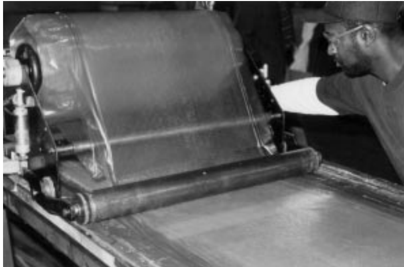
Figure 5-45 Prepreg Ply of E-Glass is Rolled Out on Consolidation Table by Composite Ships [author photo]
