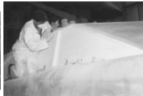
Figure 5-9 Detail Construction of a Deckhouse Plug at Heisley Marine [author photo]
