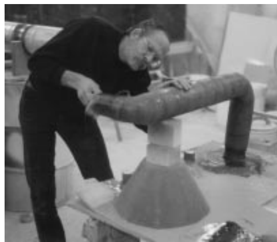
Figure 5-21 Complex Part is Prepped for Secondary Bond at Westport Shipyard [author photo]
