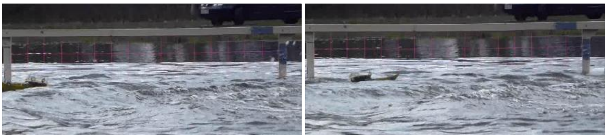
Figure 80 Snapshots of video from test run 2; pictures (left – downward pitch; right – upward pitch) show how the bow (or more correctly: forward heading end) visibly plunges and then climbs as the waves hit its lee side.
