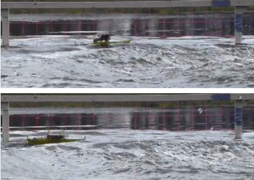
Figure 82. Snapshots of video from test run 3 showing consecutive stances of pitching downwards (bottom) and then upwards (top).
