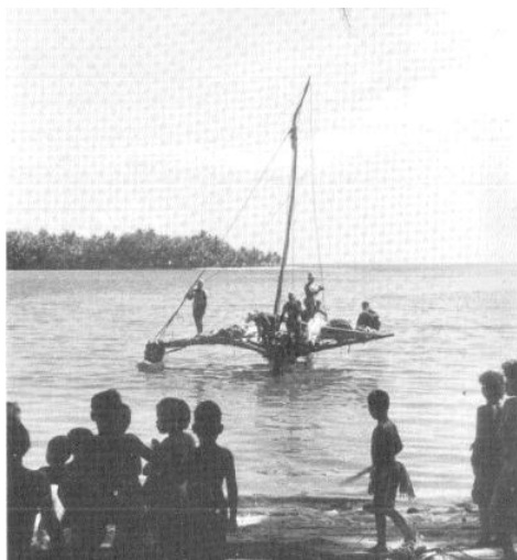
Figure 66. A sailing canoe, showing the outrigger (left) and lee platform (right) on opposite sides (from Gladwin 1970: 73).
