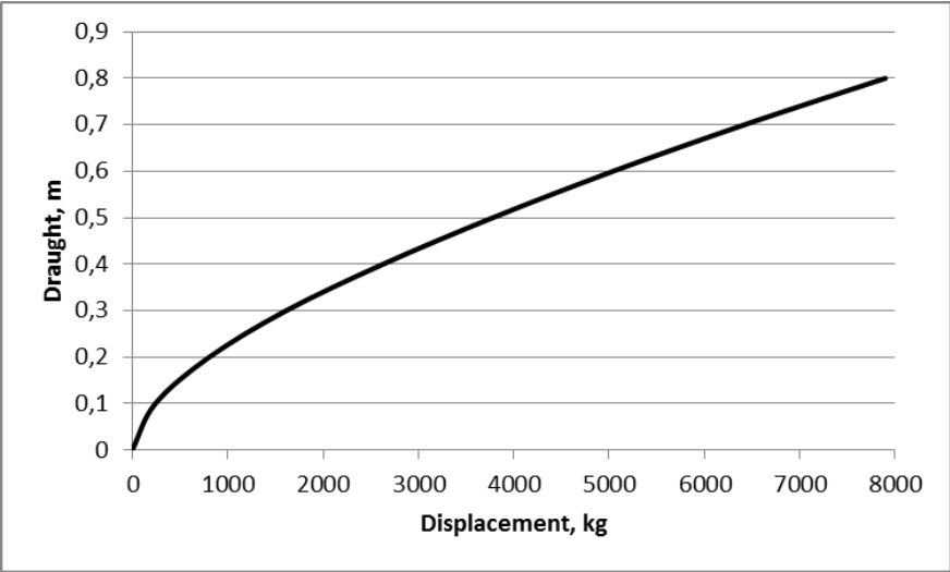
Figure 106. Diagram showing displacement (kg) against draught (m)
