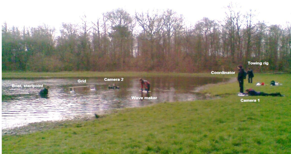
Figure 17. The test setup. The boat was towed between the two persons at the start point and camera 2 (Photo: Bo Ejstrud).
