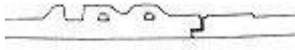
Figure 29. The box scarf connecting the two planks of the keel (from Wright 1990).
