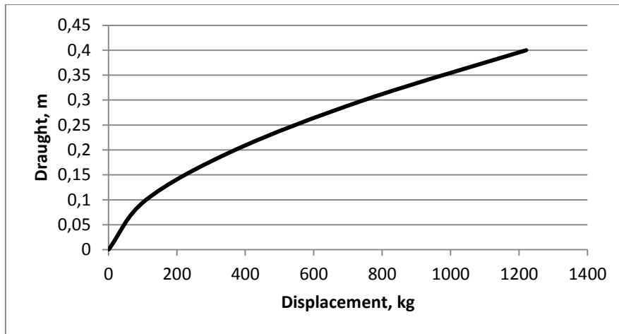
Figure 53. Singapore Sampan, displacement curve.
