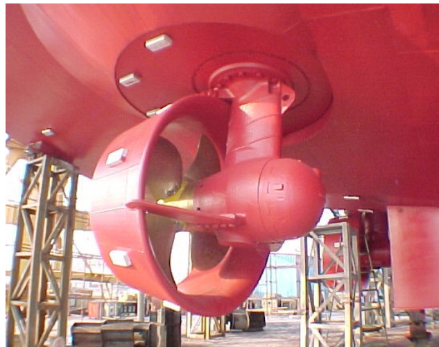
Figure 1 Ducted azimuth thrusters (Kawasaki Rexpeller KST-180).
