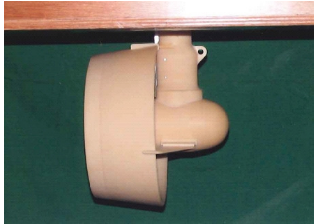
Figure 5 Test equipment using small waterproof dynamometer inside gear case housing.
