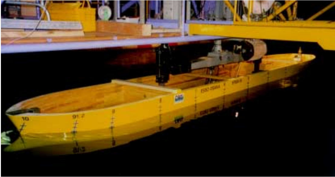
Figure (5.3) Static rudder test.
