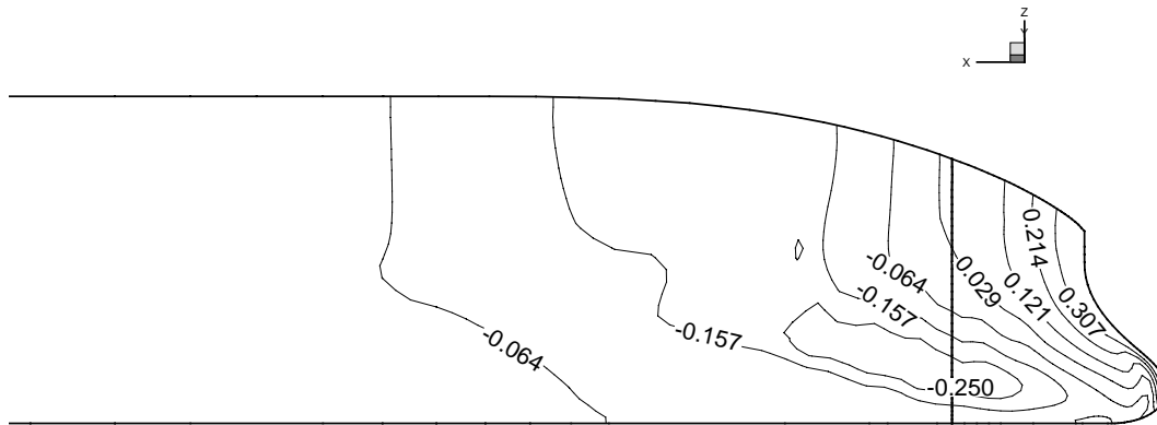
Figure (13.7) Pressure distribution on hull in the fore end of the ship.
