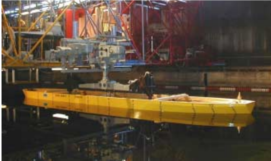
Figure (5.2) Model mounted in the PMM below the carriage.
