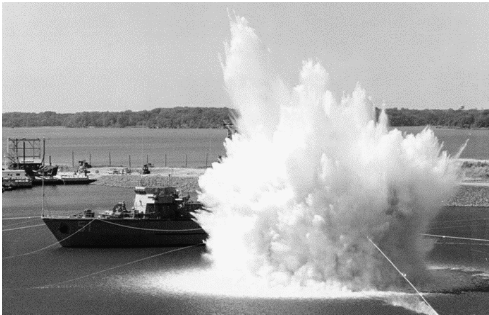
Fig 3.1. Minehunter during shock test (USS OSPREY)
