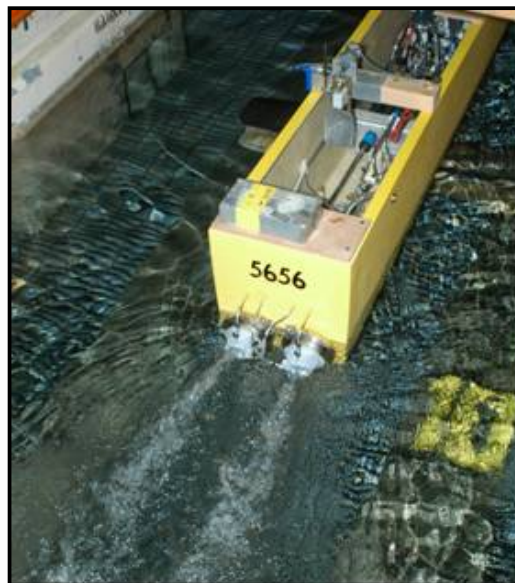
Figure 11: Self-Propulsion Model in the Towing Tank
