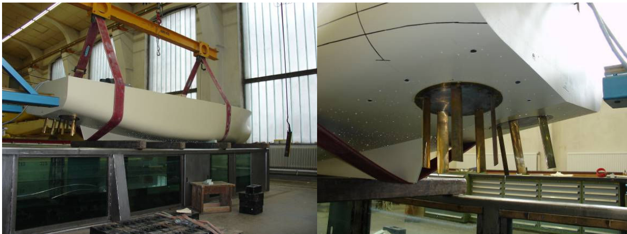
Fig. 11: Ship model and position of the pressure sensors
