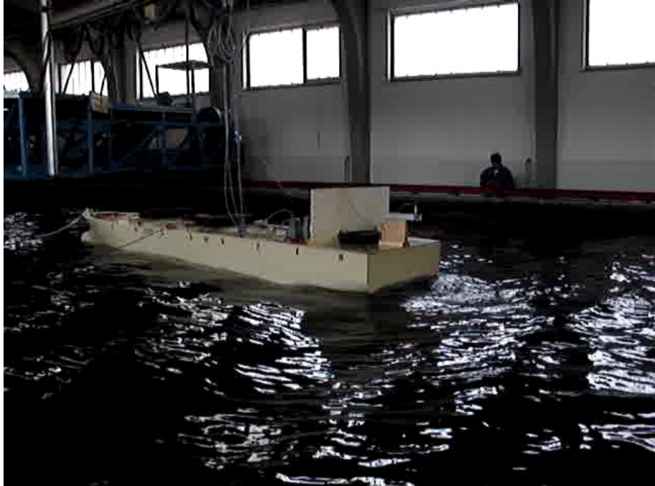
Fig. 10: Testing of stern slamming for a OSV under DP conditions
