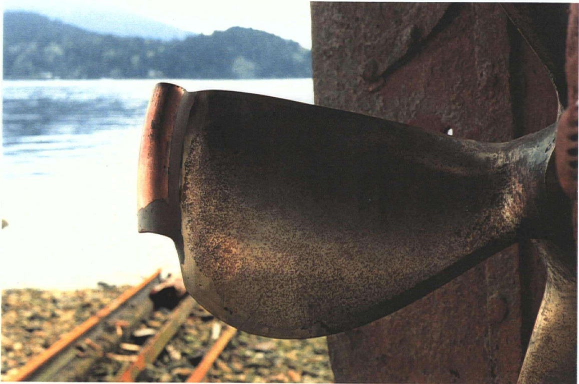
Figure 2.6 Details of the ducted tips: Seen in proportion to the rest of the blade.
