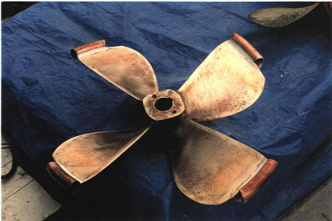
Figure 2.4 The ducted tip propeller.
