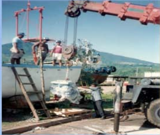
Medium size fishing travelers build in Ferro cement. Deck and inboard engines.
