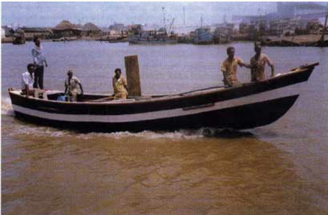
A FRP Beach Nava built by the APFC boatyard with the BOB Drive
