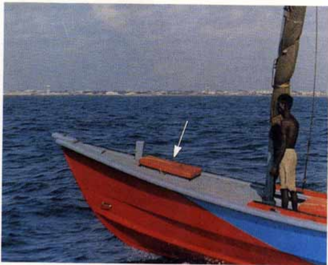
The arrow indicates the hatch through which the BLC crew shelter beneath the deck
