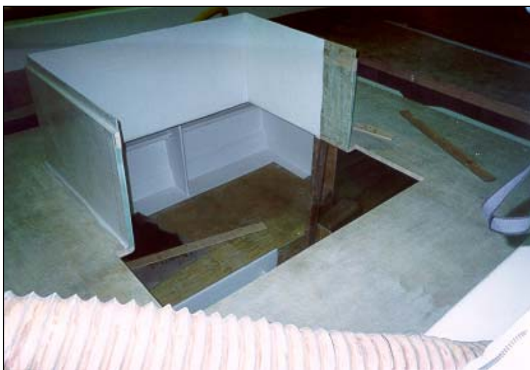
Figure 9: Construction of hatch coaming.
