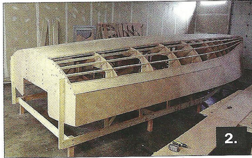
1 —Construction of the first Didi 950 started with a computer numerically controlled (CNC) cut backbone, 9mm-plywood bulkheads, and doublers interlocking. 2 —Solid longitudinals let into the bulkheads support the plywood hull skins. 3 —In way of the chine radius, the hull is skinned with two layers of cold-molded plywood strips laid transversely. 4 —The completed faired hull awaits its epoxy coatings before being turned upright.
